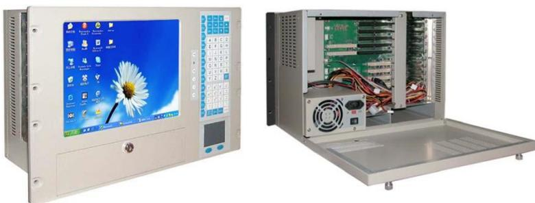
19" 7U 10 Slots 12.1" TFT LCD Workstation Chassis
