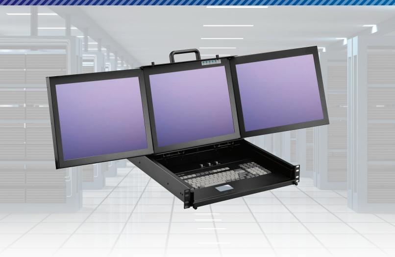
3U rackmount drawer with an integrated keyboard drawer and 3x 17" LCD monitors. These monitors have high contrast ratios (500:1). They fold away to fit into 3U rack space.
